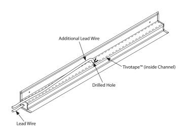
**Step 6:** Run wiring to Power Supply and connect wiring runs to Transformer. See Installation Instructions for the variety of Tivotape™ being installed for more information.
