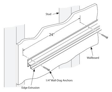
**Step 2:** Fasten Edge Channel to wall using Wall-Dog™ Screws (by others). Review the following charts for maximum allowable load capacities for this lighting system.
