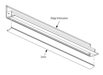
Step 2: Starting at one end of the Channel, press the side of the lens until it snaps into place. Continue pressing the lens down while sliding your hand along the lens to finish pressing it into place along the length of the Channel.
